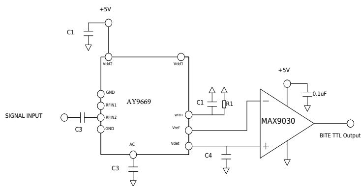
This circuit is used for system self-check, resistor R1 sets the threshold power, when the input signal is higher than the threshold power, the comparator MAX9030 outputs TTL high level. R1 setting range: 51Ohm~5.1KOhm.
