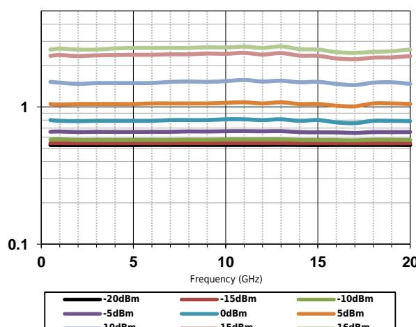
Detection voltage (V) vs. input power
