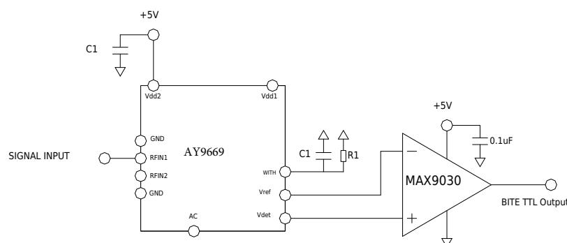
This circuit is used for system self-check, resistor R1 sets the threshold power, when the input signal is higher than the threshold power, the comparator MAX9030 outputs TTL high level. R1 setting range: 51Ohm~5.1KOhm.
