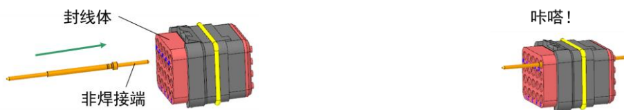
Figure 8 Installation of contacts
